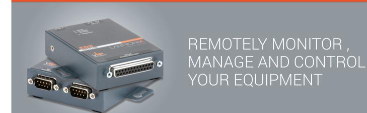
The EDS1100 and EDS2100 device servers are unique, hybrid Ethernet terminal/multiport device servers which allow remote access to and management of virtually any IT/networking equipment or edge device such as medical equipment, POS terminals or security equipment.
