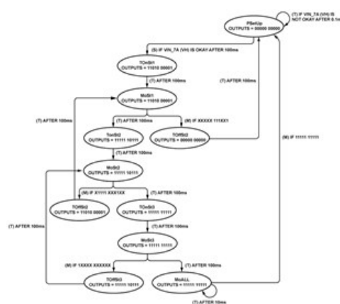
Figure 8. Power Monitor and Sequencing Control Strategy State Machine Diagram
