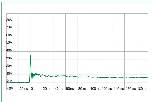
ISO10605 Contact Discharge Plot at +8 kV
