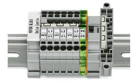
Continuous jumpers (2002 Series) readily connect an endless number of terminal blocks to each other via single jumper slot. Use the second jumper slot for additional commoning or testing.
