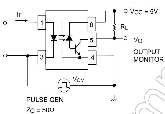
$$CM_H = \frac{320(V)}{t_r(\mu s)}, \quad CM_L = \frac{320(V)}{t_f(\mu s)}$$
