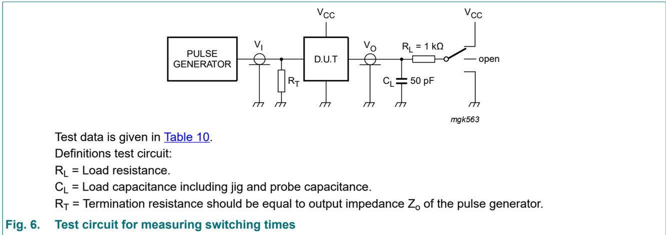
Fig. 6. Test circuit for measuring switching times
