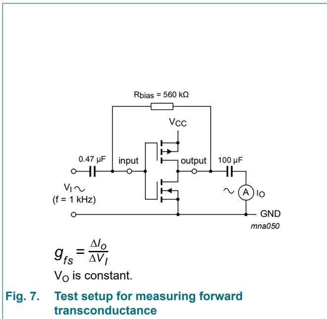
Fig. 7. Test setup for measuring forward transconductance
