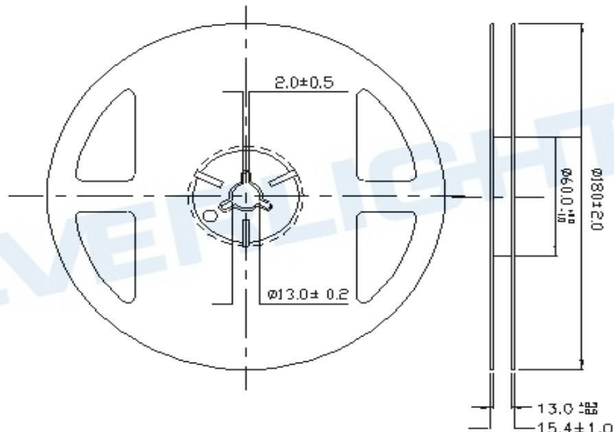
**Carrier Tape Dimensions: Loaded Quantity 800 pcs Per Reel**
