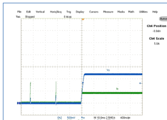
Figure 37: Short Circuit Recovery, Ch2: V_o , Ch4: I_{out}(2A/Div)
