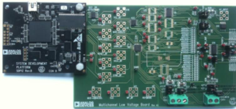
The **EVAL-AD8403SDZ** evaluation board is designed to help customers quickly prototype new **AD8403** circuits and reduce design time. The EVAL-AD8403SDZ incorporates several test circuits to evaluate the **AD8403** performance.
