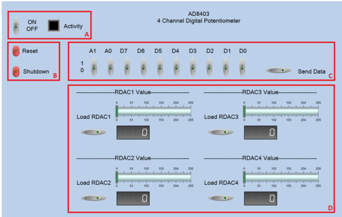
**Section A** is used to activate the board and monitor activity. The communication with the board is activated / deactivated by toggling the **ON/OFF** switch. The **Activity** LED turns green when the communication is active. If the **ON/OFF** switch is set to **ON** and the **Activity** LED is **BLACK** it means that there is a communication problem with the board.
