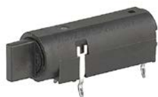
Closed fuseholder 5 x 20 mm horizontal with finger grip captive fuse carrier
