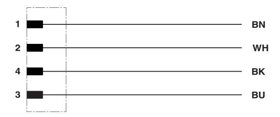
Contact assignment of the M12 connector
