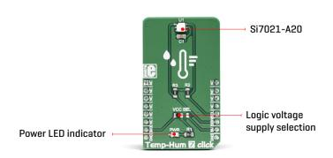
Each sensor contains the factory calibration data in the internal non-volatile memory, so there is no need for additional calibration steps. The datasheet of the Si7021-A20 offers conversion formulas, which should be used to convert the readings from the sensor to physical values, expressed in %RH and °C.
