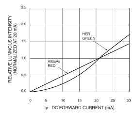
Fig. 2 Relative Luminous Intensity vs.
