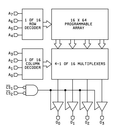
FIGURE 3. Logic diagram.
