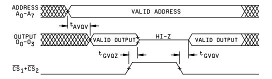
FIGURE 5. Switching waveforms.
