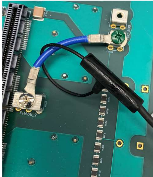
Figure 42: Shorting wire and Rogowski coil to measure short-circuit current
