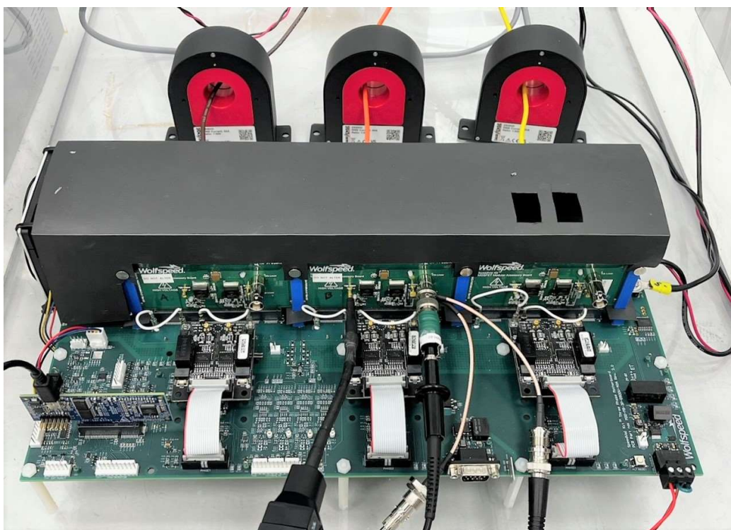
Figure 48: Three-phase SpeedVal™ Kit setup as inverter driving resistive load
