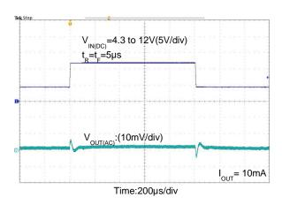
Load Transient Response  $V_{\text{OUT}}$ =3.3V
