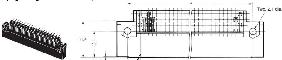
XH2A-□□42-A (Right-angle DIP Terminals with Fastening Pins)
