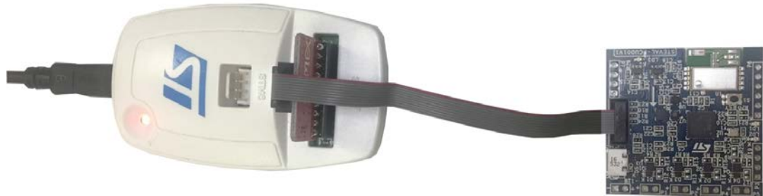
Figure 6. ST-LINK/V2 connected to the STEVAL-FCU001V1 evaluation board via adapter
