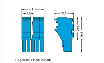
Female connector, 2022 Series, Push-in CAGE CLAMP®
