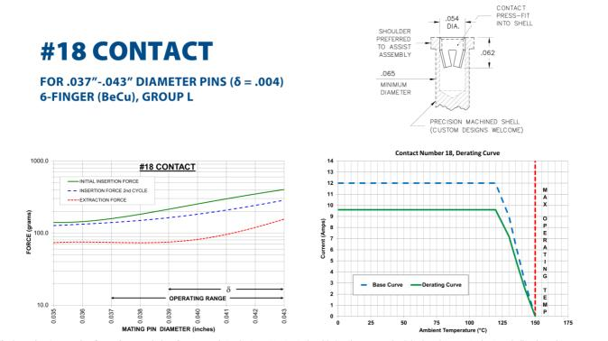
The insertion / extraction force characteristics above were derived using a 30 microinch gold-plated contact and polished steel gauge pins having a bullet-shaped tip. The curves represent typical average values; they are best used to compare the differences between similar size contacts and to guide you in selecting one that is suitable for your application. Your results may vary, so for your specification, we encourage you to obtain complimentary samples for your evaluation.
