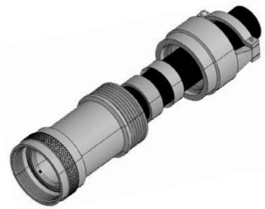
These Backshells from Amphenol not only provide the cable support and strain relief, but ensure the cable sealing and environment protection by means of high quality sealing grommet and grommet follower. The strain relief nut is tightened squeezing the grommet on to the cable jacket during assembly. These Backshells from Amphenol give 6 feet water sealing protection when used with perfectly jacketed cable and are suitable for harsh environment applications.
