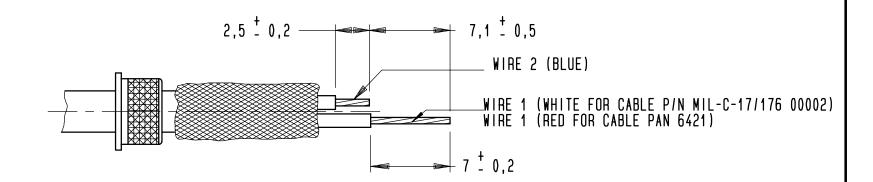
PUT THE TWO WIRES IN THE INSULATOR BUSHING UNTIL IT'S BUT AGAINST THE SHIELD BRAID, (SEE ORIENTATION) INTRODUCE THE WIRE 1 (RED) INTO THE CENTER CONTACT INTRODUCE THE WIRE 2 (BLUE) INTO THE INTERMEDIATE FERRULE
