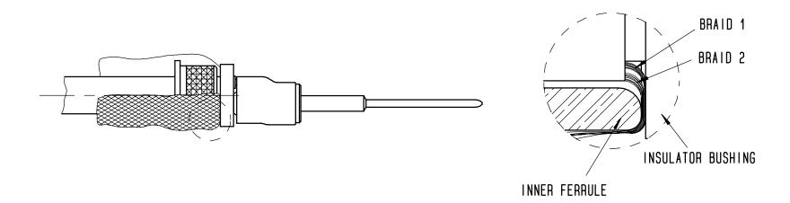
STEP 6/ PUT THE CABLE/CENTER CONTACT ASSEMBLY IN THE REAR OF THE OUTER CONTACT CUT AROUND THE BRAID SO THAT THE BRAID IS FLUSH WITH THE SURFACE OF THE OUTER CONTACT CRIMP THE OUTER CONTACT IN THE INDICATED CRIMPING AREA USING:
