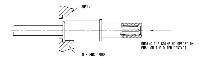
STEP 7/INSPECTION DIMENSIONS AFTER CRIMPING
