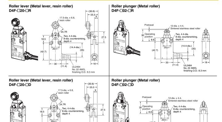
Note: Each dimension has a tolerance of 0.4 mm unless otherwise specified.
