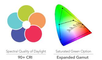
**HIGHEST QUALITY TUNABLE WHITE LIGHT:** Lumenetix-araya recreates daylight by mixing LED colors of the rainbow – red, amber, mint, cyan and blue, plus green if an expanded gamut option with saturated green is desired – to deliver full spectrum light from 1650K to 8000K at 90+ CRI.
