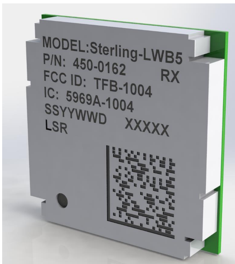
Figure 1 Sterling-LWB5 Base SIP Module (450-0162)
