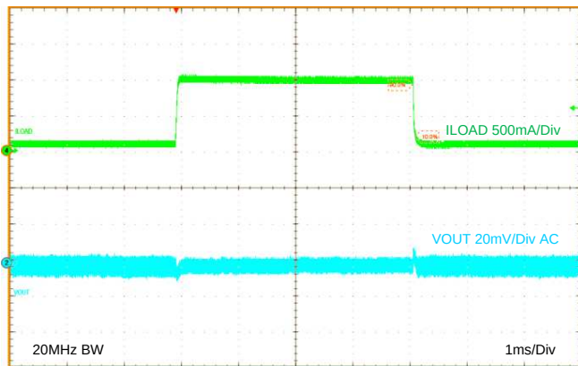
Figure 60. Load Transient V_{OUT} = 3.3\text{ V}
