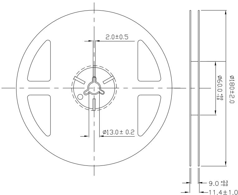
Note: The tolerances unless mentioned is  $\pm 0.1\text{mm}$ , Unit = mm
