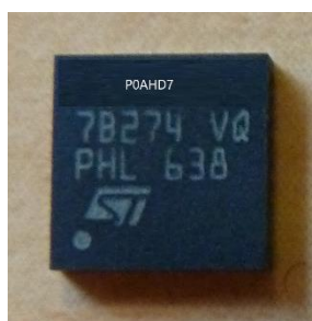
Figure 14: Picture of the Cryptographic Module (VQFN32) – Marking P0AHD7
