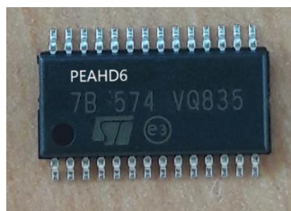
Figure 11: Picture of the Cryptographic Module (TSSOP28) – Marking PEAHD6
