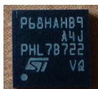
Figure 6: Picture of the Cryptographic Module (VQFN32) – Marking P68HAHB9
