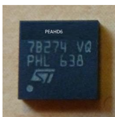
Figure 12: Picture of the Cryptographic Module (VQFN32) – Marking PEAHD6
