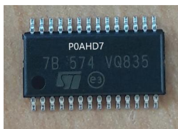
Figure 13: Picture of the Cryptographic Module (TSSOP28) – Marking P0AHD7
