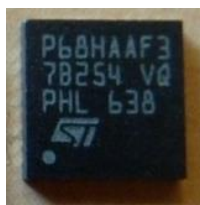
Figure 10: Picture of the Cryptographic Module (VQFN32) – Marking P68HAAF3
