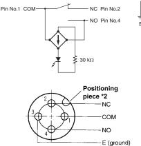
\*1. "Lit when not actuated" means that when the actuator is in the free position, the indicator is lit, and when the actuator is turned or pushed and the contact comes
