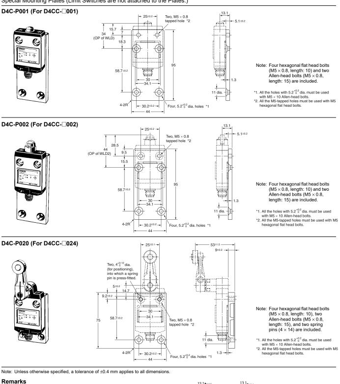
There is no difference in mounting pitch between the Mounting Plate and the WL/WL-N. The mounting depth of the D4CC with the Mounting Plate attached is, however, shorter than that of the panelmounted WL/WL-N.
