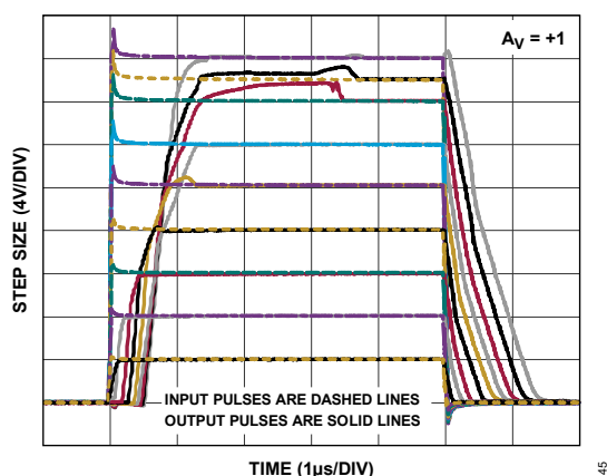
Figure 135. Large Signal Noninverting Output Behavior, Without Input RC
