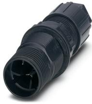
Conductor connectors, QUICKON connection, number of positions: 3+PE, 1 mm<sup>2</sup> ... 2.5 mm<sup>2</sup>, 690 V, 20 A, black, with one QUICKON nut, external cable diameter: 9 mm ... 14 mm, QUICKON fast connection
