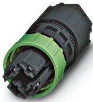
Connector, QUICKON connection, number of positions: 3+PE, 1 mm<sup>2</sup> ... 2.5 mm<sup>2</sup>, 690 V, 20 A, black, external cable diameter: 9 mm ... 14 mm
