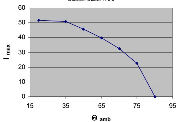
Max. allowable ambient Temp. at specific power loss
