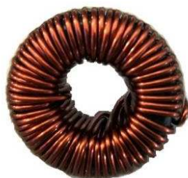
Figure 8: Inductor used for buck and boost converter
