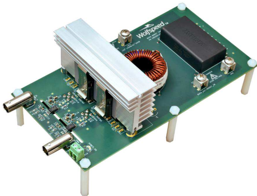
Figure 1: KIT-CRD-3DD065P/CRD-3DD12P, buck-boost evaluation kit
