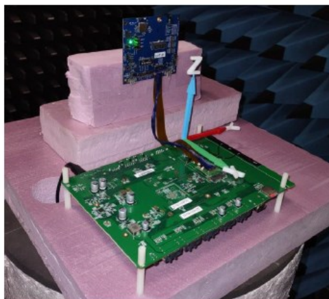
Figure 24: Sona TI351 Radiated Performance Measurement Setup
