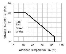
Fig. 3 FORWARD CURRENT VS. DERATING CURVE
