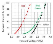
Fig. 2 FORWARD CURRENT VS. FORWARD VOLTAGE
