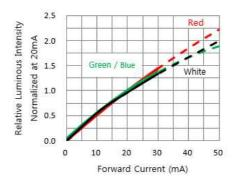
Fig. 4 RELATIVE LUMIOUS INTENSITY VS. FORWARD CURRENT
