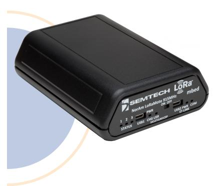
The EPM2M-NORAM Sensor Module is an industrial grade wireless sensor for LoRa based wireless sensor network technology from Semtech. LoRa is built for long range wireless sensor applications. The EPM2M-NOARM provides an easy to use, seamless connection between the physical sensing world and the EPM2M-LORA Gateway using LoRa. At the heart of the EPM2M-NORAM module is the Semtech LoRa SX1272.
