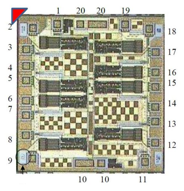
Note: Pad numbers reflect terminal numbers when placed in Case Outlines R and X (see paragraph 1.2.4 and figure 1)
