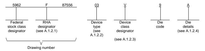
A.1.2.1 RHA designator. Device classes Q and V RHA identified die shall meet the MIL-PRF-38535 specified RHA levels. A dash (-) indicates a non-RHA die.
