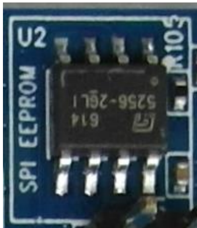
Figure 16: SPI EEPROM schematic and PCB
