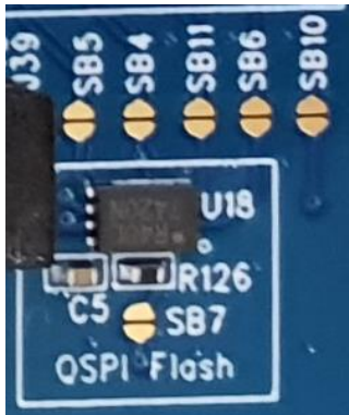
Figure 19: Optional external serial SPI flash IC (U18) schematic and PCB
