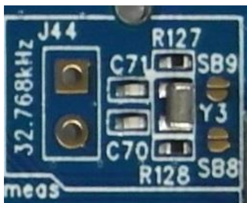
Figure 20: Optional external 32.768kHz crystal circuit schematic and PCB
