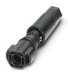
Photovoltaic connector, Range of articles: PV-C1M-S, Connector, housing material: PPE, color: black, number of positions: 1, min. conductor cross section: 2.5 mm², max. conductor cross section: 6 mm², rated current: 27 A, Connection method: Spring-cage, Type of contact: Pin. can only be released using a tool
