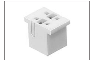
Shunt plug for 0.635×0.635 mm square contacts or 0.64 mm diameter round contacts (Double plug type) DIC-407W D-75 DIC series...15
