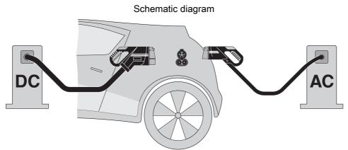
The Combined Charging System (CCS) principle - standard-compliant charging system for electric vehicles, which supports both conventional AC charging and fast DC charging. Both Vehicle Connectors fit into the CCS Vehicle Inlet.
