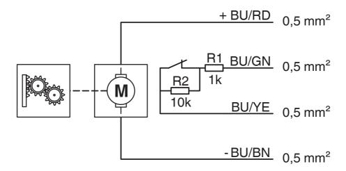
Block diagram of the locking actuator
