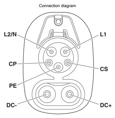
Pin assignment of vehicle charging inlets
