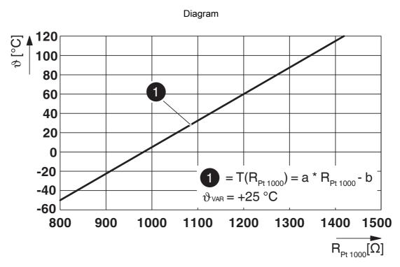
Pt 1000 characteristic curve at an ambient temperature of 25°C for temperature measurement at the DC contacts
