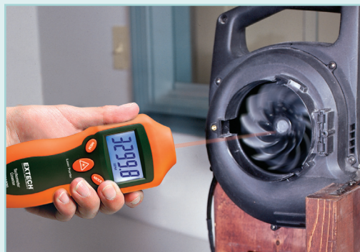
Non-contact fan blade RPM or REV testing
