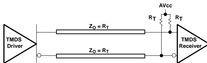
Figure 1. Termination for TMD5 Output Driver
