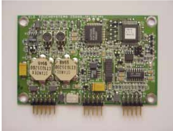
Figure 2.5 Touchscreen Cabling System for Internal Serial Controller
