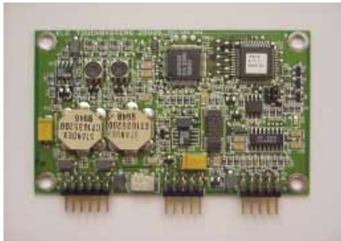
Figure 2.10 2500S Internal Serial Controller
