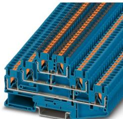
Multi-level terminal block, with equipotential bonder, nom. voltage: 500 V, nominal current: 20 A, number of connections: 6, connection method: Push-in connection, Rated cross section: 2.5 mm<sup>2</sup>, 1st, 2nd and 3rd level, cross section: 0.14 mm<sup>2</sup> - 4 mm<sup>2</sup>, mounting type: NS 35/7,5, NS 35/15, color: blue
