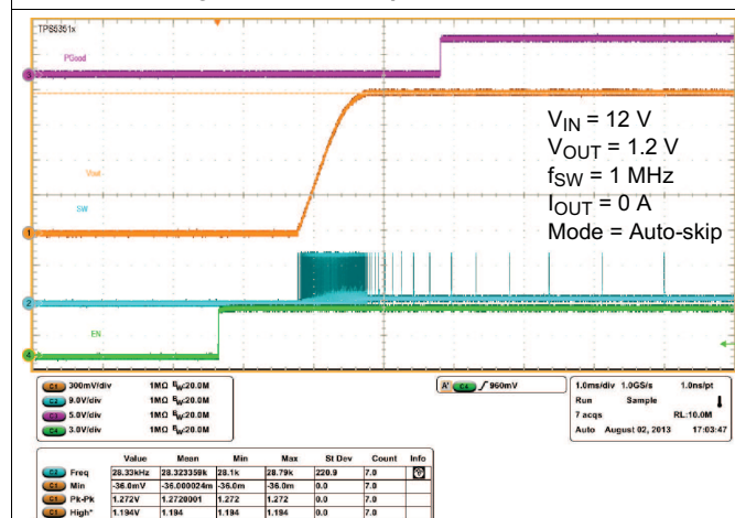
Figure 19. Auto-Skip Mode Load Transient
