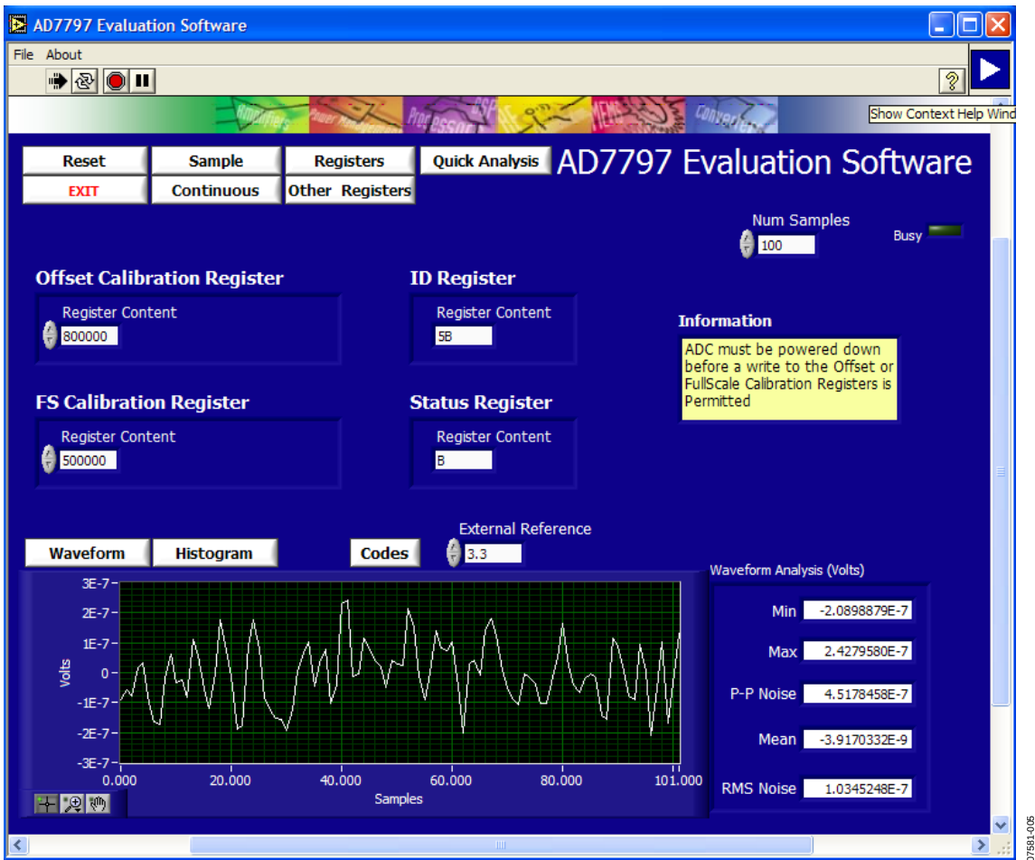
Figure 5. AD7797 Evaluation Software Other Registers Window
