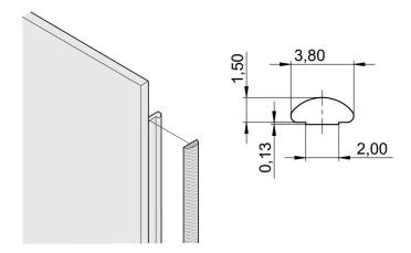
The textile EMC gaskets are inserted into a slot on the right hand side of the U-shaped front panels. The gaskets are glued to the front panel.
