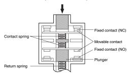
Conforms to EN60947-5-1 Direct Opening Operation ⊖
