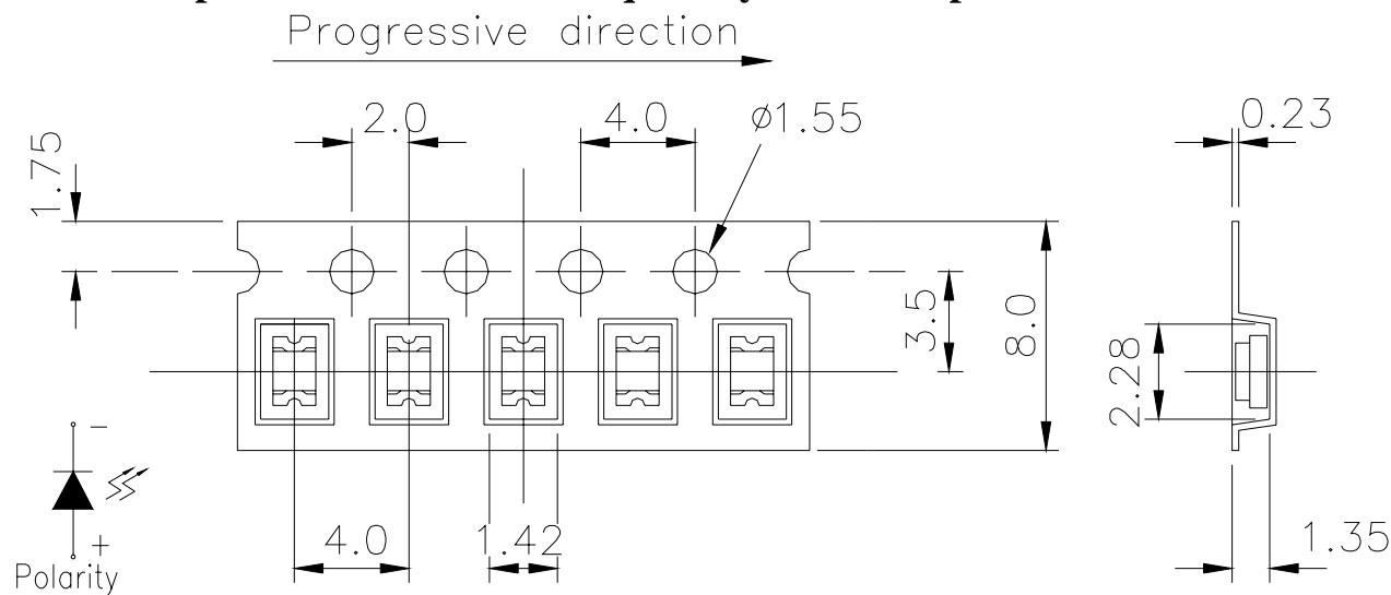
**Note:** The tolerances unless mentioned are  $\pm 0.1$ , unit = mm.
