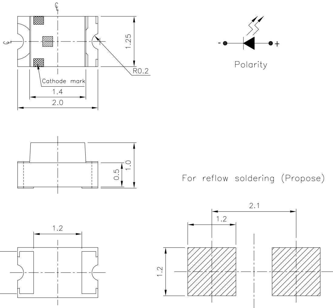
**Note:** The tolerances unless mentioned are  $\pm 0.1$ , unit = mm.
